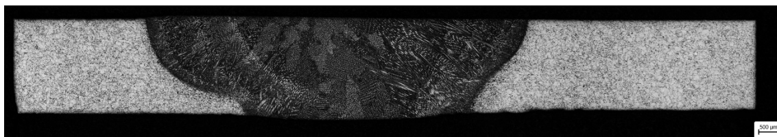
HAYNES® 233® 0.125" sheet manual GTAW with HAYNES® 233-W® filler metal
