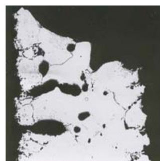
alloy 600 Average Metal Affected = > 22 Mils (560 µm)/Side
