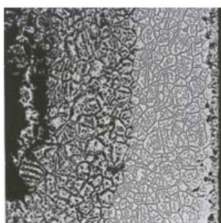
INCONEL alloy 601 Average Metal Affected = > 22 Mils (560 µm)/Side
