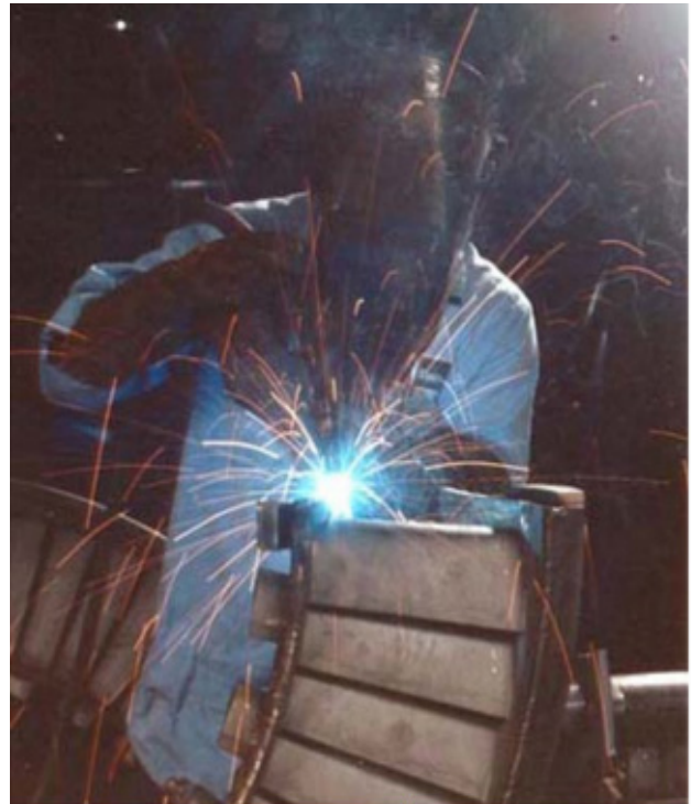
556 alloy upgrades MULTIMET® alloy stator vanes in industrial turbines.
