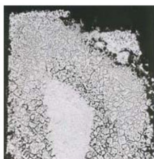
HASTELLOY® X alloy Average Metal Affected = > 22 Mils (560 µm)/Side
