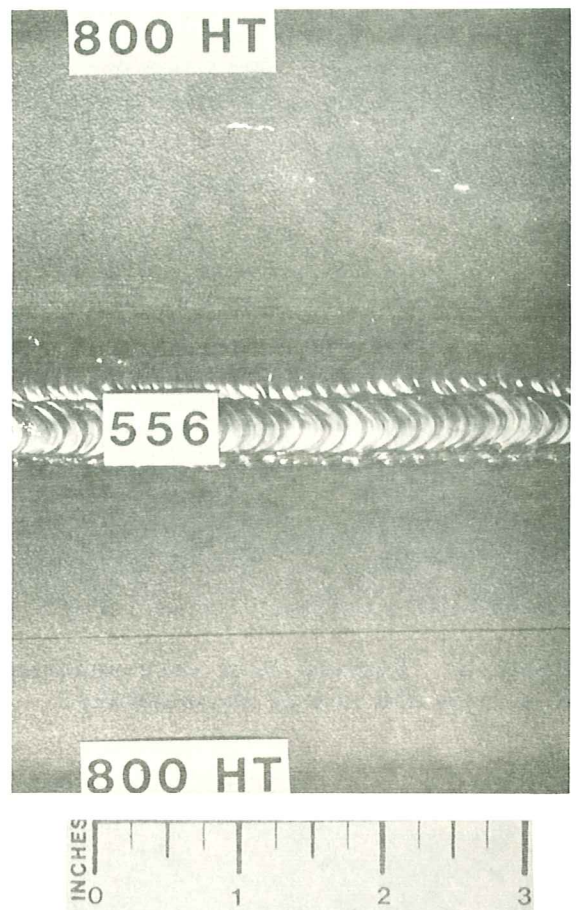
FIGURE 3: Weldment consisting of 1/2-inch thick alloy 800HT plates gas-tungsten-arc welded using alloy 556 filler Metal (800HT/556/800HT).
