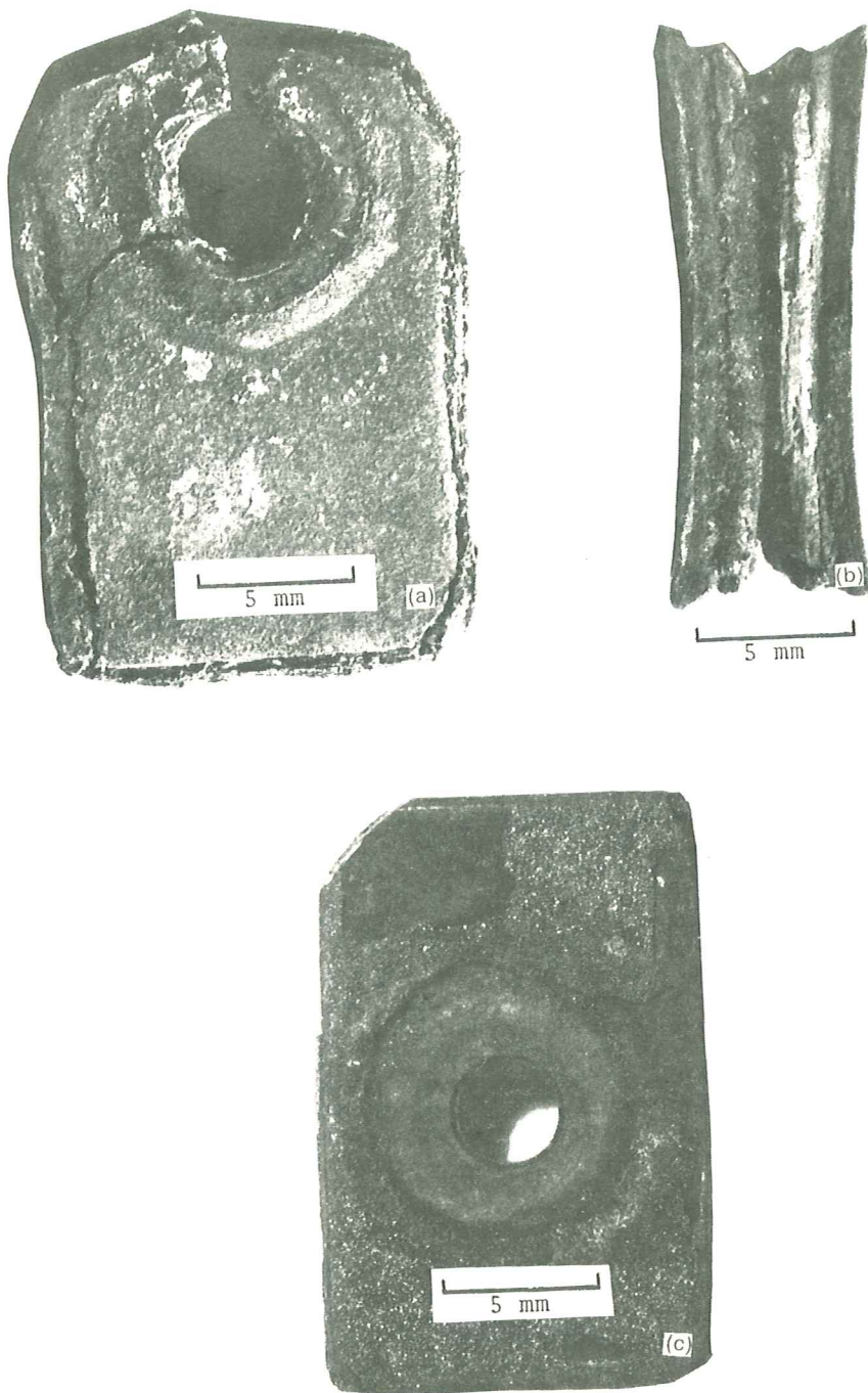
Figure 2 - Coupons after testing in molten salt at 900°C, (a) Cabot 214 in hydroxide for 3.5 days, (b) Hastelloy S in carbonate for 21 days, and (c) Hastelloy X in carbonate for 21 days.
