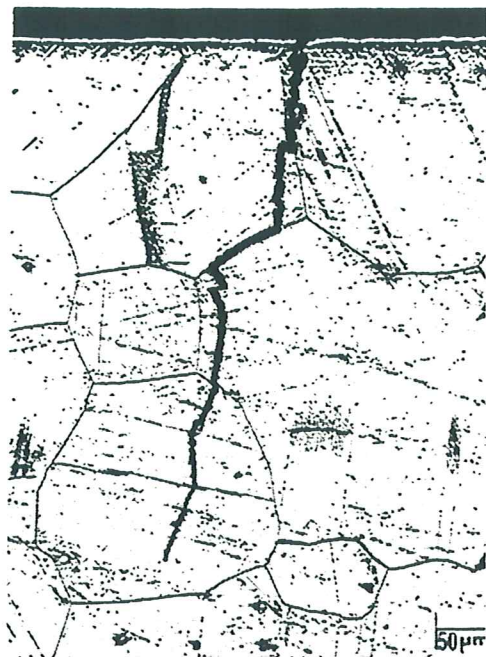
FIG. 7.2: OPTICAL PHOTOMICROGRAPH OF ALLOY 617 (SAME SPECIMEN AS IN FIG. 7.1) SHOWING MIXED MODE SECONDARY CRACK PROPAGATION AND MICROSTRUCTURE; ETCHED.
