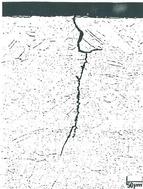
FIG. 6 OPTICAL PHOTOMICROGRAPH OF ALLOY X, FATIGUE TESTED AT 982°C (1600°F) \Delta\epsilon_t = .4\% , SHOWING SECONDARY CRACKING AND MICROSTRUCTURE; ALSO NOTICE OXIDATION ON THE SURFACE; ETCHED.
