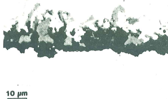
Fig. 5 - Optical photomicrographs showing the chromium oxide scale with chromium sulfides formed on top of the oxide scale for HR-160 alloy tested at 700°C (1292°F) for 500h. The specimen was nickel-plated prior to mounting.
