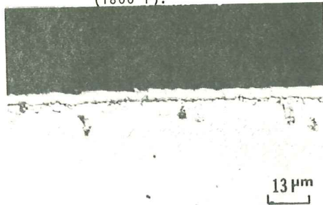
Figure 2: Optical photomicrograph showing a carbide scale formed on the alloy X sample tested at 982°C (1800°F) for 55 hours.
