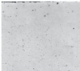
HAYNES® 214® alloy Average Metal Affected = 1.8 mils (45.7 µm)
