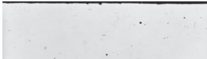
HAYNES® 214® alloy Average Metal Affected = 0.5 mils (13 \mu\text{m} )
