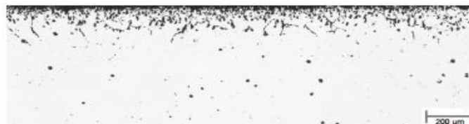
RA330® alloy Average Metal Affected =8.7 mils (221 \mu\text{m} )
