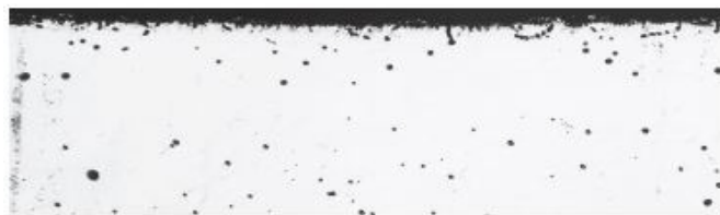
Alloy 600 Average Metal Affected =4.8 mils (122 \mu\text{m} )
