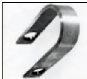
HASTELLOY ® B-3 ® alloy Annealed + 1 hour at 700°C (No cracking, 24 hours)
