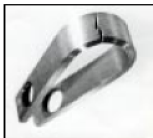
HASTELLOY ® B-2 alloy Annealed + 1 hour at 700°C (Intergranular cracking, 3 hours)
