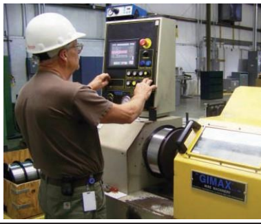
The GIMAX Precision Winder produces high-quality layer wound welding spools.
