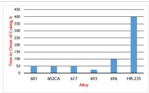
**Time to Onset of Coking (in Accelerated Metal Dusting Tests)**
