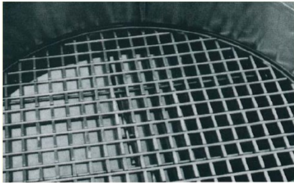
Nitric acid catalyst grid support made from HAYNES ® 230 ® alloy and plate bar. Excellent creep strength at 1700°F (925°C) makes the alloy highly suitable for this application.
